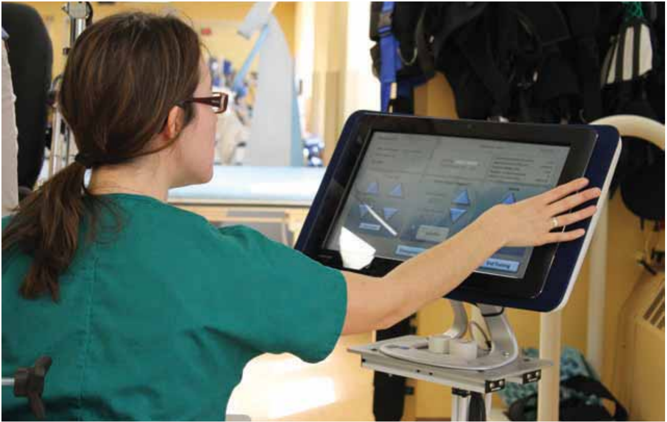
Therapist Jennifer Matuszewski programs a body-weight support system. The system is designed to allow the amount of body-weight support to be easily adjusted throughout the session.
